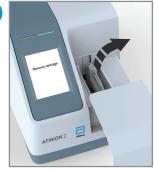
Remove and immediately discard the used test cartridge. Close the lid manually when the analyzer is not in use.
