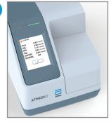
Record the result when it appears on the screen. Touch to accept. The lid opens automatically.
